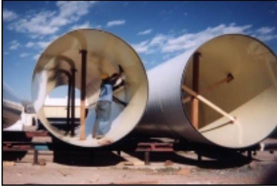
108" Spiral Weld Steel Pipe manufactured by Thompson Pipe and internally lined with Madison's Corropipe II PW for Denver Water.
