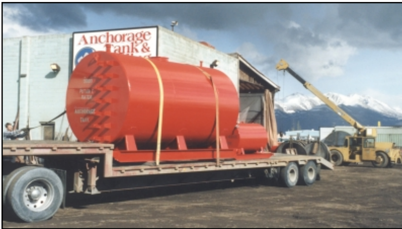
Potable water tanks lined with Corrocote II PW leaving Anchorage Tank in Alaska.
