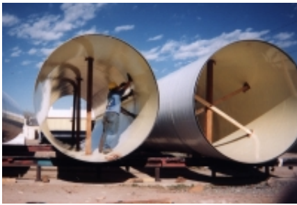
Spiral Weld Steel Pipe manufactured by Northwest Pipe and internally lined with Madison's CorroPipe II PW®
