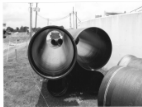
Fig. 3 Polyurethane lining after 6 year exposure in the same yard
