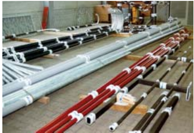
Powder coating adds extra durability and corrosion protection to these hot-dip galvanized utility poles, which were powder coated immediately after galvanizing and then packaged for shipping. Instead of field painting, many products are galvanized and painted in the shop prior to installation.
