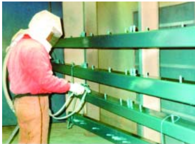
When steel is painted, as with these beams, the paint provides barrier protection to the base steel. The integrity of a duplex system relies on the proper application of a uniform paint coating to properly-prepared hot-dip galvanized steel.
