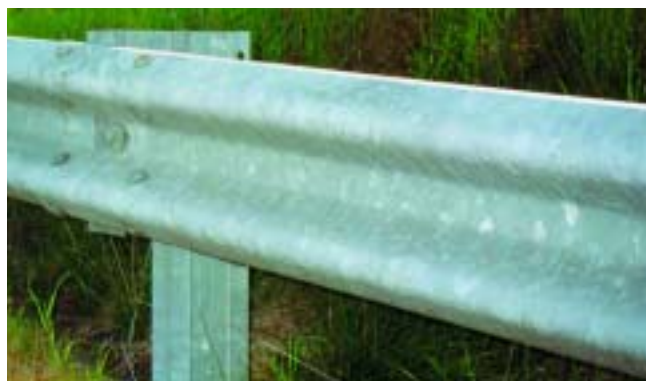
Newly galvanized steel (above) typically exhibits a bright, shiny appearance. Weathered galvanized steel (below) usually possesses a dull, mottled gray appearance. Different ages of galvanized steel require different surface cleaning and profiling prior to painting.
