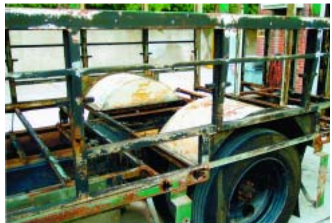
This painted trolley bus frame exhibits extensive corrosion on its entire framework.
