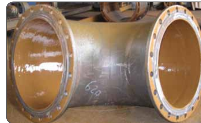
A section of pipe, showing the beautiful glossy finish provided by Madison's CorroPipe II TX-15.
